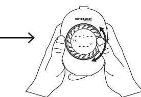
Rotate the main button counter clockwise (past 00:00) to delete the setting. The remaining time periods will rearranged in order.
