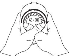
Rotate the main button 90° clockwise while holding the main button down.
