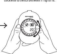
Rotate the main button clockwise or counter clockwise to increase or decrease the time with 30 minutes. (00:00 to 23:30).
