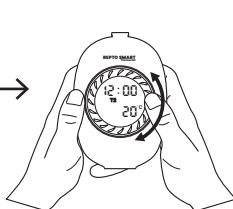
Rotate the main button clockwise or counter clockwise to switch between T1 up to T8.
