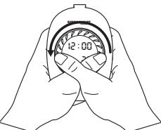
Rotate the main button 90° counter clockwise while holding the main button down.
