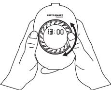
Rotate the main button clockwise or counter clockwise to set the hour.
